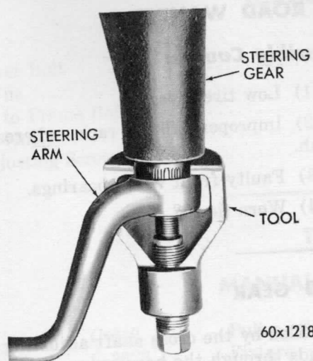
Fig. 3—Removing Steering Gear Arm (Typical) (Tool C-3646)
